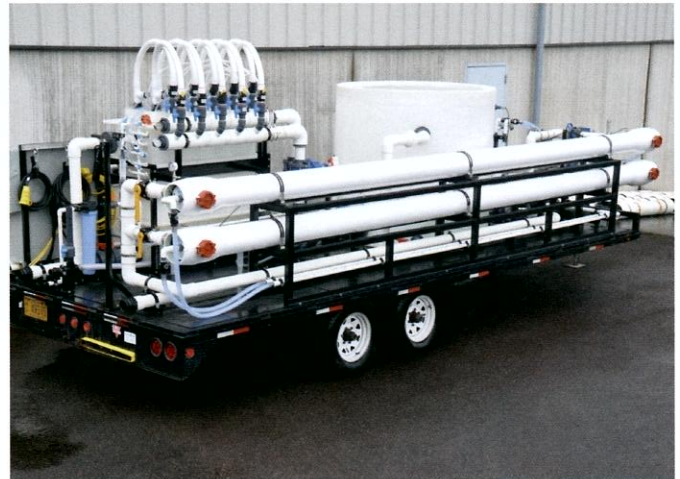
A sewer mining forward osmosis pilot unit manufactured by Hydration Technology Innovations, LLC
