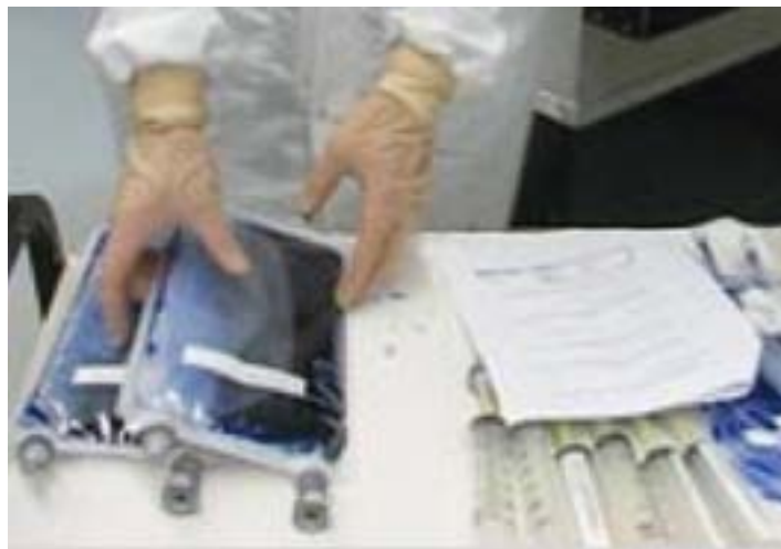
NASA's Forward Osmosis Test Packs
