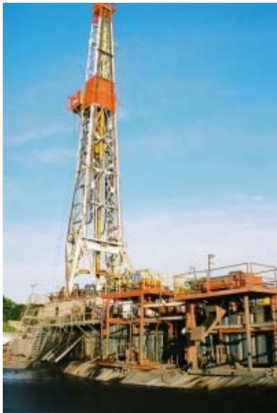
Drill beside produced water containment pit, photo courtesy of the Produced Water Society
